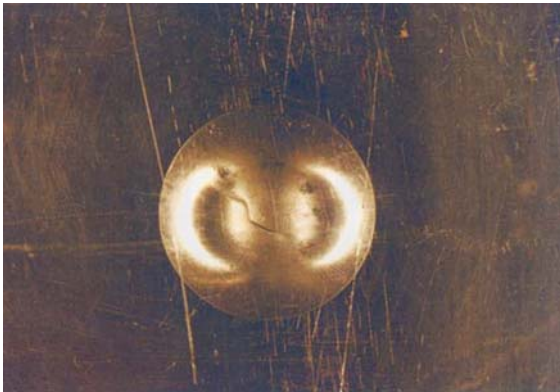
Fig. 5 The deformed specimen after performing the Erichsen test on aluminum sheet using nylon as lubricant
